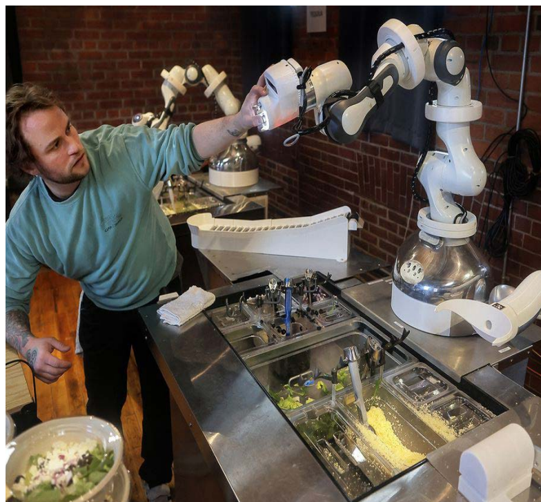
"Alfred" is a food safe-certified robotic arm that can sit in front of a row of hotel pans of ingredients and can hold traditional kitchen utensils like scoops and tongs. Photo courtesy Lane Turner/ Boston Globe
