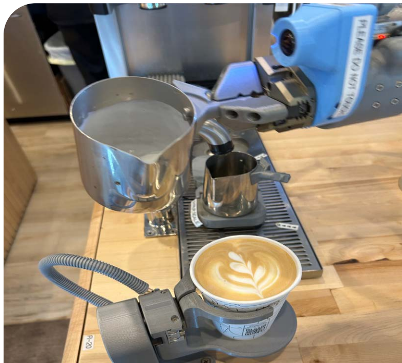
The Arty Barista Bot uses deep learning-based visual inspection to monitor drink quality at each step to ensure a perfect cup with every order. Photo courtesy Kathleen Stoehr
