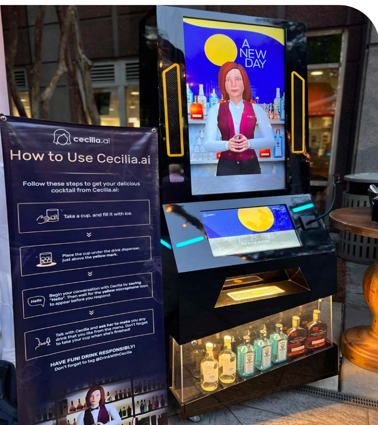
(Left) Cecilia.ai is an interactive bartender where guests interested in a drink can come up and tell it their order. Cecilia.ai can respond to the order, such as saying a certain ingredient isn’t available or suggesting an alternative option. Cocktails are also available on a touchscreen menu, and the drink is delivered through a slot in the machine. Photo courtesy Cecilia.ai
