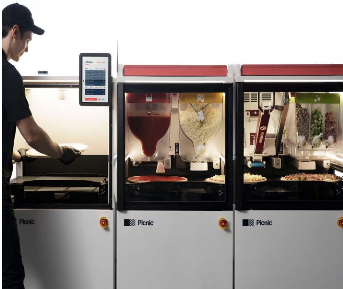
Picnic Works' Picnic Pizza Station is an automated, robotic back-of-house makeline that allows one person to make up to 100 consistent pizzas an hour, while reducing food waste to around 2%. Photo courtesy Picnic Works
