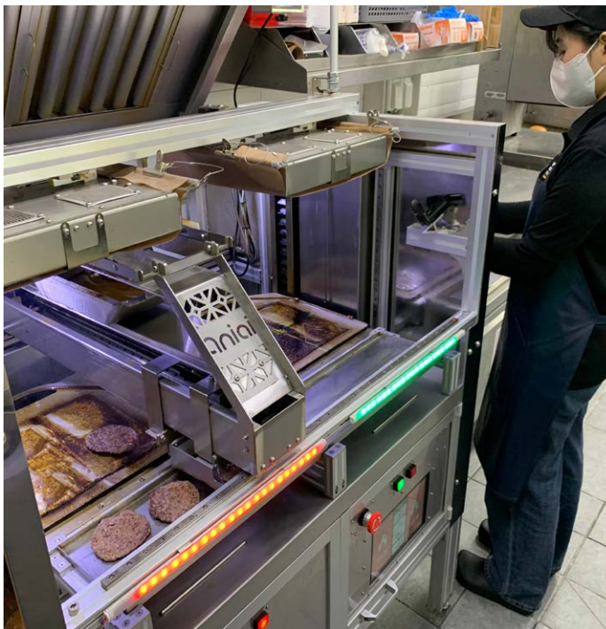
Aniai's flagship product, Alpha Grill, is designed to cook hamburgers easily, efficiently, and with consistent quality. Featuring a double-sided grill design and a rapid cooking system, the Alpha Grill is able to cook eight perfect burger patties in under a minute. Alpha Grill is packed with AI components to check and control food quality. With an intuitive touch-screen monitor, users can customize cooking conditions, access real-time quality metrics, operational stats, inventory data, and more. Photo courtesy Aniai
