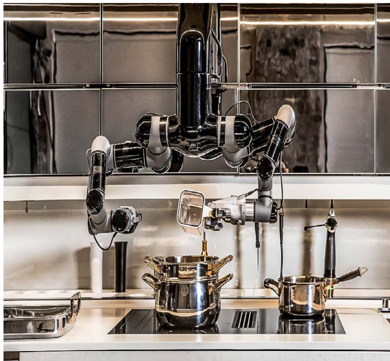
Moley Robotics’ robotic kitchen features a dexterous robot integrated into a luxury kitchen that prepares freshly-cooked meals at the touch of a button. At the heart of the new technology are two robotic arms featuring fully-articulated “hands” that can reliably reproduce the movements of human hands. Photo courtesy Moley Robotics
